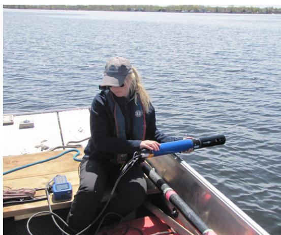
Using a multi parameter sonde to measure water quality.
